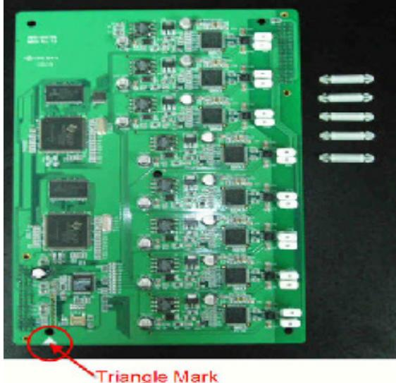
d.)Module 1 (the 9~6th port of FXS/ FXO) Must be put in the extension 1 area. Please insert in the extension 1 area of regular posts 5 inside in a regular hole.
